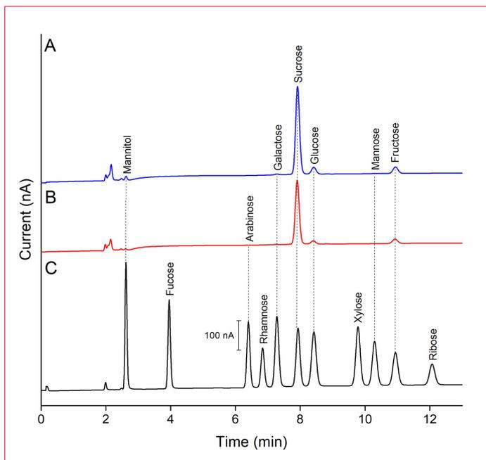
**Figure 8.** Overlay of chromatograms obtained from 3  $\mu\text{L}$  injections of [A] intact green coffee beans from India (blue curve), [B] crushed green coffee beans from India (red curve), and [C] 10  $\mu\text{M}$  standard mix containing 11 carbohydrates in ultrapure water (black curve).
