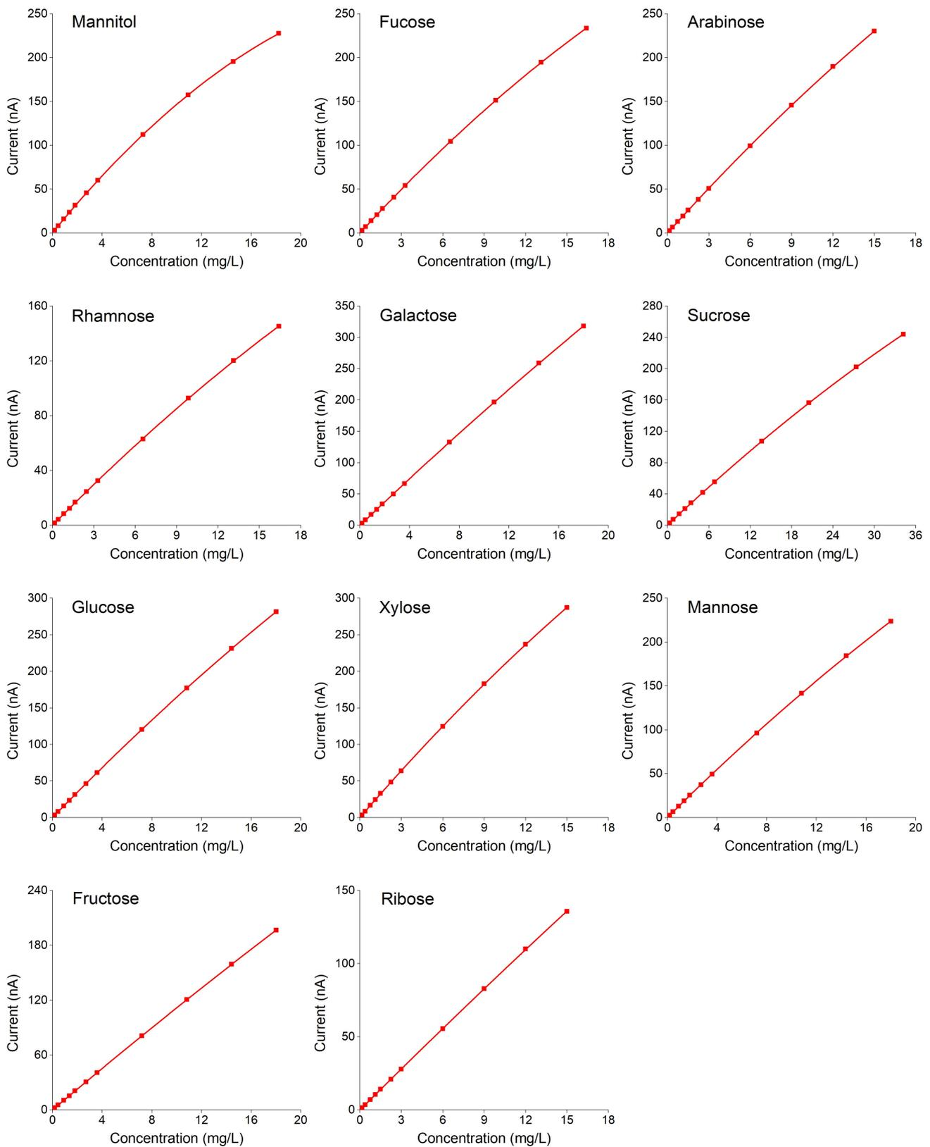
**Figure 3.** Calibration curves of the 11 sugars in the range of 0.2 - 18.2 mg/L for mannitol, 0.2 - 16.4 mg/L for fucose and rhamnose, 0.2 - 15.0 mg/L for arabinose, xylose, and ribose, 0.2 - 18.0 mg/mL for galactose, glucose, mannose, and fructose, 0.3 - 34.2 mg/L for sucrose. A quadratic fit was applied for all sugars, were the origin was ignored and a weight factor of  $1/\text{concentration}^2$  was used.
