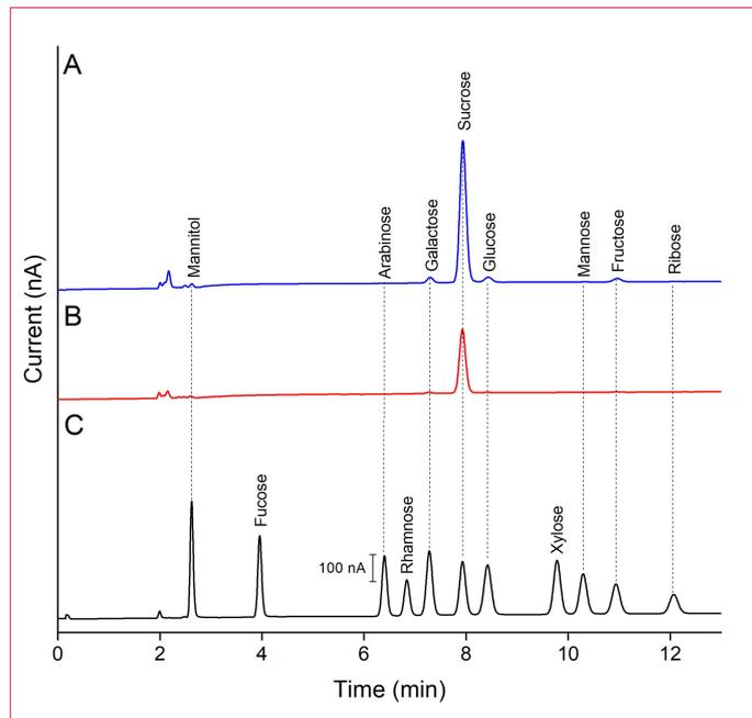
**Figure 9.** Overlay of chromatograms obtained from 3  $\mu\text{L}$  injections of [A] intact green coffee beans from Guatemala (blue curve), [B] crushed green coffee beans from Guatemala (red curve), and [C] 10  $\mu\text{M}$  standard mix containing 11 carbohydrates in ultrapure water (black curve).
