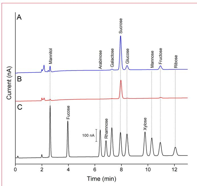
**Figure 10.** Overlay of chromatograms obtained from 3  $\mu\text{L}$  injections of [A] intact green coffee beans from Ethiopia (blue curve), [B] crushed green coffee beans from Ethiopia (red curve), and [C] 10  $\mu\text{M}$  standard mix containing 11 carbohydrates in ultrapure water (black curve).
