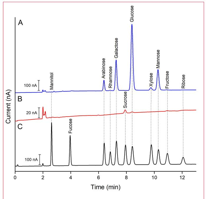
**Figure 7.** Overlay of chromatograms obtained from 3  $\mu\text{L}$  injections of [A] instant coffee sample #4 - total carbohydrate determination (blue curve), [B] instant coffee sample #4 - free carbohydrate determination (red curve), and [C] 10  $\mu\text{M}$  standard mix containing 11 carbohydrates in ultrapure water (black curve).
