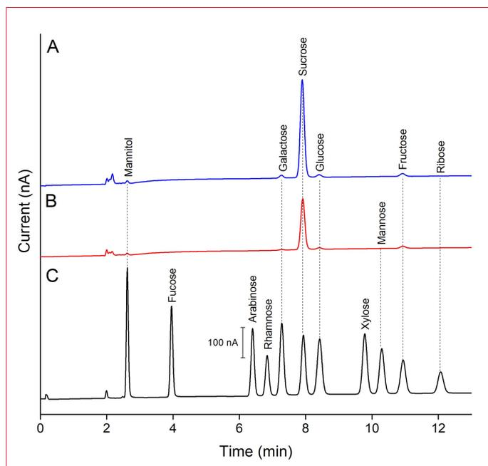
**Figure 11.** Overlay of chromatograms obtained from 3  $\mu\text{L}$  injections of [A] intact green coffee beans from Brazil (blue curve), [B] crushed green coffee beans from Brazil (red curve), and [C] 10  $\mu\text{M}$  standard mix containing 11 carbohydrates in ultrapure water (black curve).
