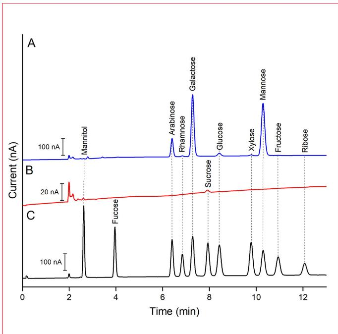
**Figure 6.** Overlay of chromatograms obtained from 3  $\mu\text{L}$  injections of [A] instant coffee sample #3 - total carbohydrate determination (blue curve), [B] instant coffee sample #3 - free carbohydrate determination (red curve), and [C] 10  $\mu\text{M}$  standard mix containing 11 carbohydrates in ultrapure water (black curve).
