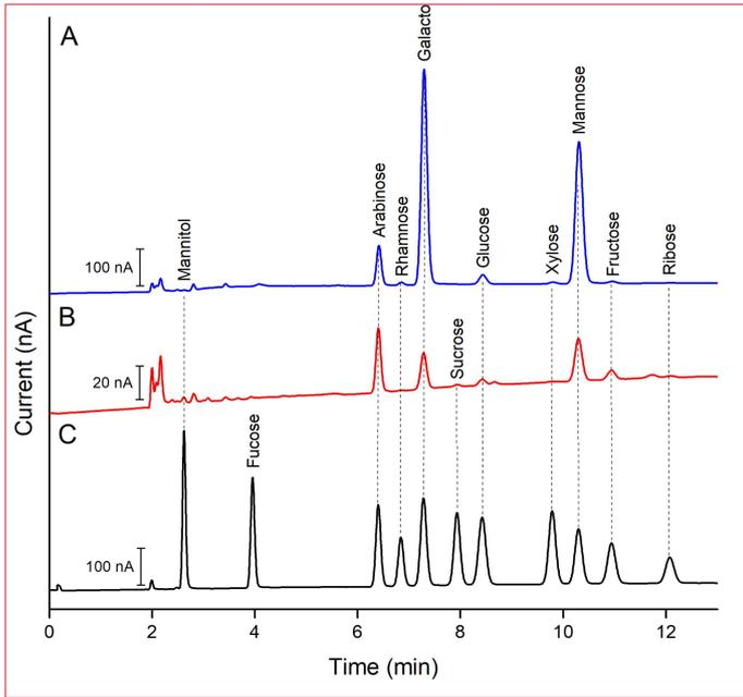
**Figure 4.** Overlay of chromatograms obtained from 3  $\mu\text{L}$  injections of [A] instant coffee sample #1 - total carbohydrate determination (blue curve), [B] instant coffee sample #1 - free carbohydrate determination (red curve), and [C] 10  $\mu\text{M}$  standard
