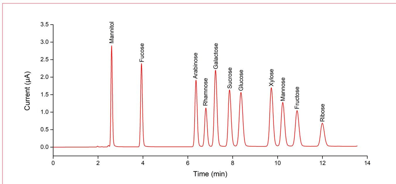
**Figure 2.** Chromatogram obtained from a 3  $\mu\text{L}$  injection of 100  $\mu\text{M}$  carbohydrate standard mix containing galactose, fructose, glucose, sucrose, mannitol, fucose, arabinose, rhamnose, xylose, mannose, and ribose in ultrapure water.
