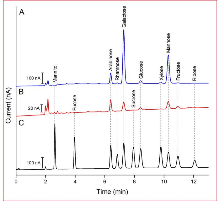
**Figure 5.** Overlay of chromatograms obtained from 3  $\mu\text{L}$  injections of [A] instant coffee sample #2 - total carbohydrate determination (blue curve), [B] instant coffee sample #2 - free carbohydrate determination (red curve), and [C] 10  $\mu\text{M}$  standard
